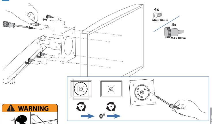
WARNING! Stored Energy Hazard: The arm mechanism is under tension and will move up rapidly, on its own, as soon as attached equipment is removed. For this reason, DO NOT remove equipment unless the arm has been moved to the highest position! Failure to follow this instruction may result in serious personal injury and/or equipment damage!
